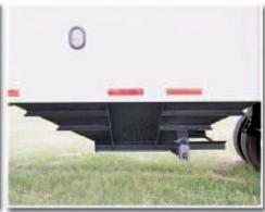
The hoppers on Maurer steel grain trailers are built to receive a retrofit side discharge chute. Anytime during the life of your trailer you can order a chute and add it to your trailer.
