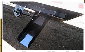
Side chute with extension shown. Chute extends 2" past side of trailer. Also shown is optional 2—speed gear reducer
